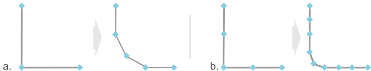
Figure 4.8: Longer faces provide less control when subdivided.
